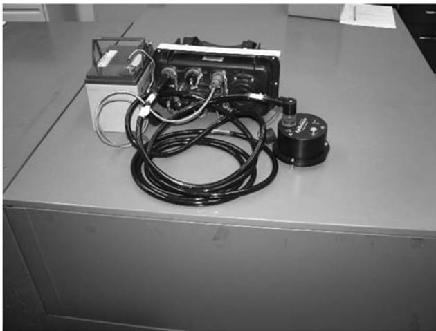
**Figure 2.** The IRIS/PASSCAL broadband stations used in this project consisted of an Episensor accelerometer and an RT-130 recorder, powered by a 12 volt battery. (Any use of trade names is for descriptive purposes only and does not imply endorsement by the U.S. government.) These units were housed in steel security boxes bolted to the floors in small alcoves.
