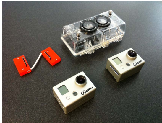
Fig. 1. GOPRO Cameras with stereo housing and synchronization cable.
