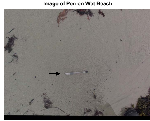
Fig. 5. One of a pair of stereo camera images used for initial in-air testing of the system's ability to generate dense 3D point clouds. Here a pen was laid on a sandy beach to further test the resolving capability of the method.
