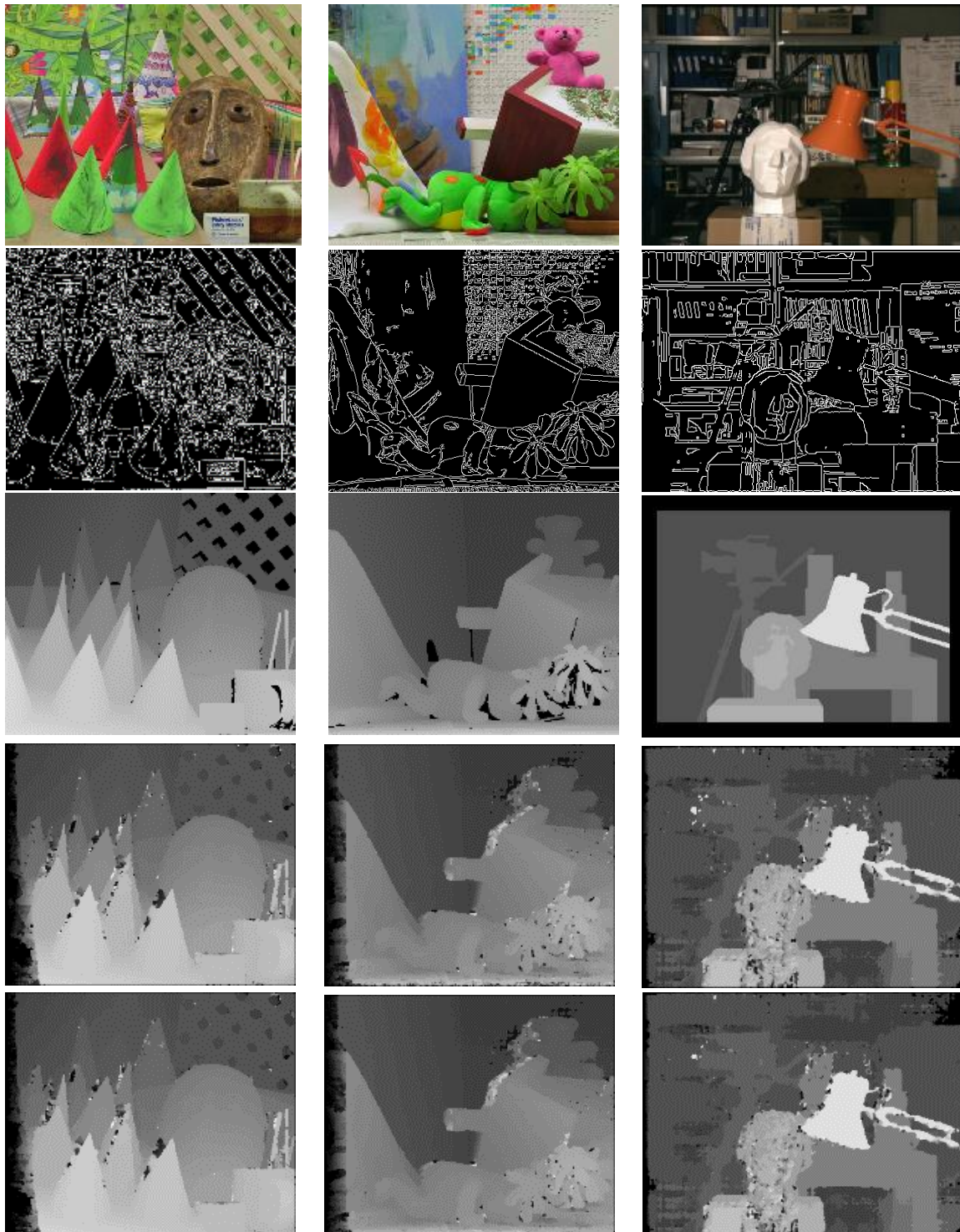
Figure 2 Experiment Results. Top to bottom row: image, Canny edges, ground truth, SGM depth map and depth map obtained by the reported algorithm.
