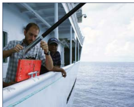
CCOM/JHC grad student Kevin Jerram adjusts the position of a calibration target below OKEANOS EXPLORER's EK60 fisheries echosounder.
