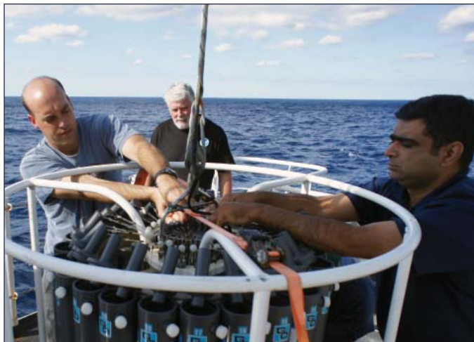
Tom Weber (left) and Mashkoor Malik (right) get ready to deploy a CTD rosette aboard OKEANOS EXPLORER.
