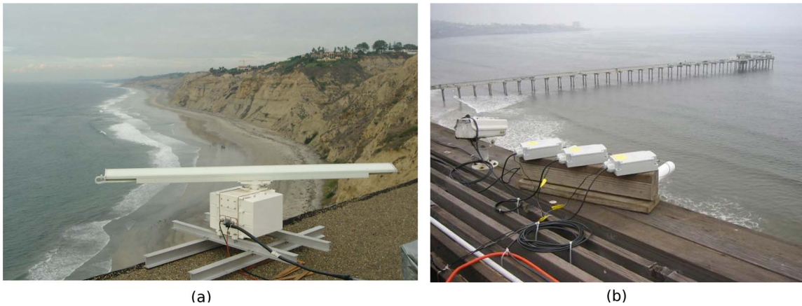
Fig. 2. Instrument deployment during NCEX on the roof of the SWFSC building in La Jolla, Ca. (a) Image of La Jolla Black's beach in the background looking North with the X-band vertically polarized scanning radar deployed by UMass in the foreground. (b) Ohio State University video cameras in foreground and SIO pier in the background.
